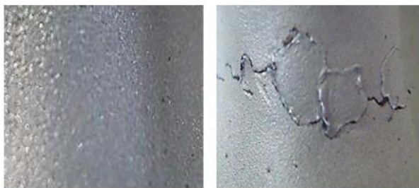
Fig. 4: Mold surface change over (Left: Before, Right: After) several vulcanizations
